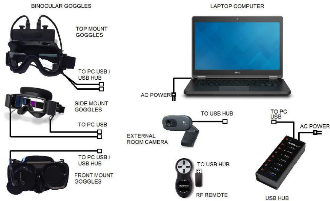
Figure 3.6.2 Laptop PC connection diagram
